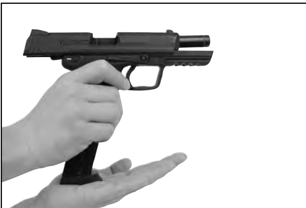
Operation of magazine release using the index finger of the firing hand
