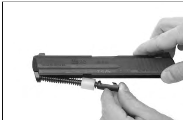
Insert the recoil spring guide rod
