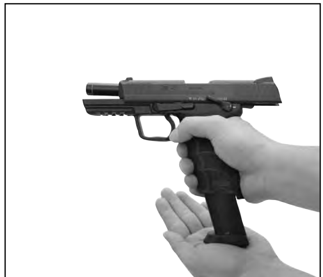
Operation of magazine release using the thumb of the firing hand
